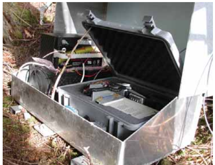
Remote acoustic recording station ("Orcabox") at Langara Island Photo: John Ford
